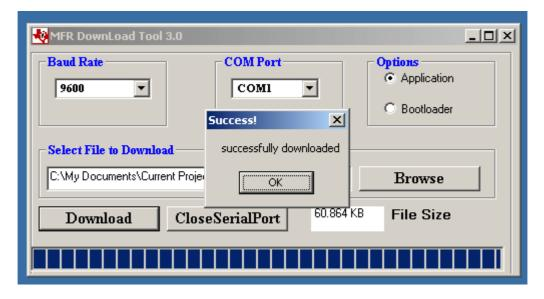
The tool should display a message box that indicates that the download was successful. At this point the module will exit the Boot loader Application and start the new Target Application. Also notice that the tool displays the size of the file it just finished downloading.
